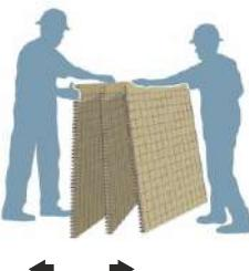
2. Stand the unit upright with the stapled row at the top. Two men each grasp an end panel and together open the unit out in the desired direction. The unit will unfold and be self-supporting. Pull the unit out to its full length and ensure it is in the correct position.
