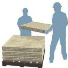
1. Two workers place a Mil unit on the ground horizontally in the location in which the wall is to be erected.
