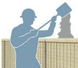
8. Place 12" – 18" of fill material in the bottom of the end cells, either manually or using appropriate loading equipment, such as a front loader. This helps to anchor the units. Ensure fill material is always placed in the center of each cell.
