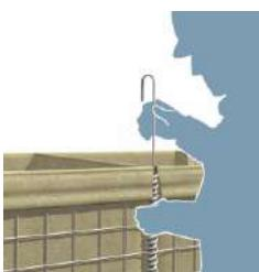
5. Insert a joining pin down the center of both the front and back overlapped corner coils, thus joining them together. Ensure the pin is fully fitted.
